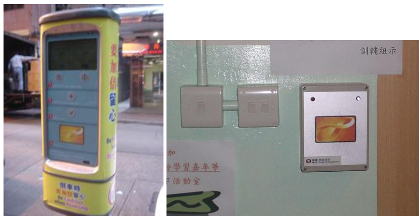
Fig. 4: Octopus terminals at a parking meter (left), and as a classroom attendance tracker (right)
