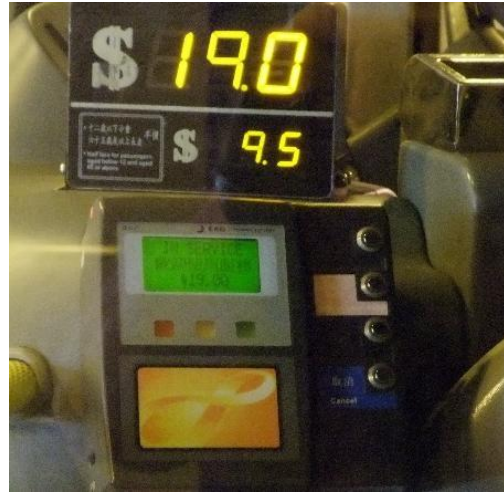
Fig. 5: Octopus reader on a bus showing cost of fare and remaining card credit
