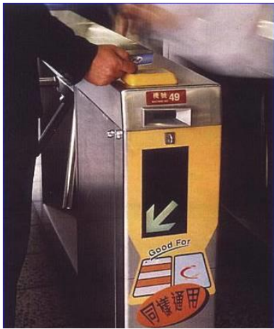
Fig. 6: A customer waving an Octopus card over a card reader mounted on a subway turnstile
